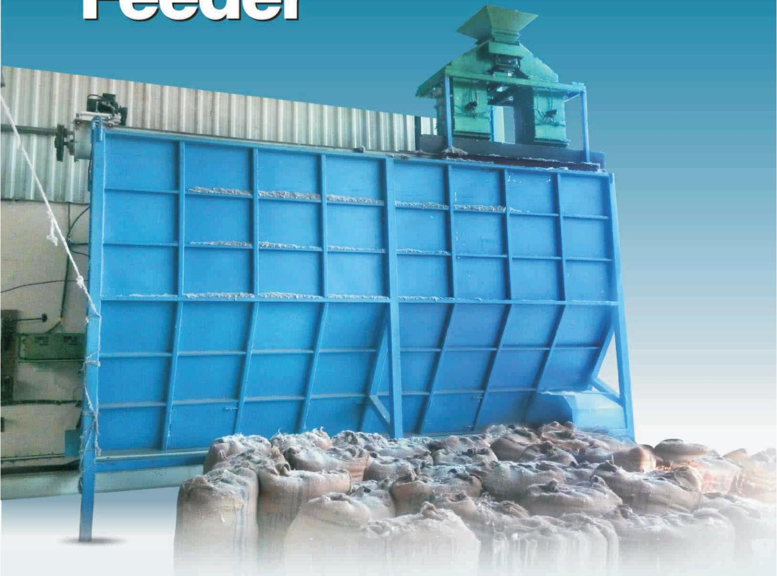
**This system is used for uniform and continuous feeding of Cottonseeds to the oil mills.**
